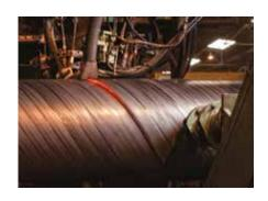
Two spiral mills feature the latest welding and ultrasonic technology for the manufacture of spiral welded pipe. The mills conform to the highest specifications required by leading water, oil and gas customers.
